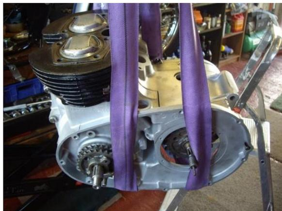
Engine assembled and ready to be lifted into frame
