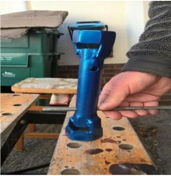
A major issue I had was to find a 1 ½ in box spanner to tighten up the final drive sprocket.
